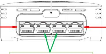
LAN4 Should be connected to the TV, connecting any other device to this port will cause the port to be disabled.
